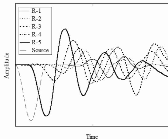
Figure 2. Source signal and receiving signals from a typical DEM S-wave propagation simulation ( $D_{50} = 2.0$  mm;  $e = 0.63$ ;  $\sigma'_3 = 150$  kPa. Note: for clarity, the amplitudes of the receiving signals are upscaled to facilitate comparison)
