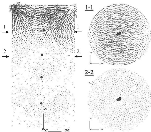
Figure 7. Particle velocity vectors on different cutting planes of a DEM specimen at a 10ms time point after excitation
