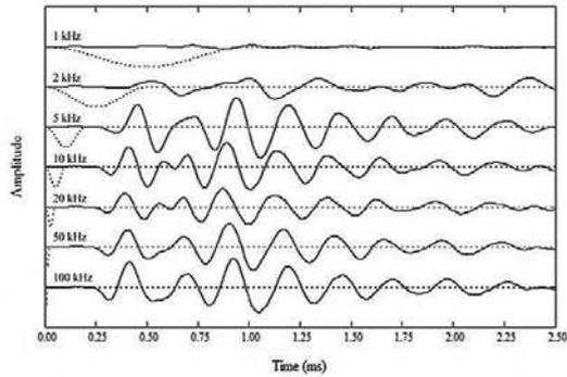
Figure 3. Response of a receiver in the time domain, excited by a sine pulse with different frequencies ( $D_{50} = 2.0$  mm;  $e = 0.63$ ;  $\sigma'_3 = 150$  kPa. Note: for clarity, the scale of the magnitude for the source signal and the receiving signals are different)
