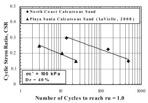
Figure 8. Comparison between North Coast calcareous sand and Playa Santa calcareous sand prepared at  $D_r$  = 40% and tested under  $\sigma_c^\prime$  = 100 kPa
