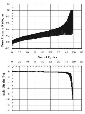
Figure 3. Typical behavior of North Coast calcareous sand subjected to cyclic loading
