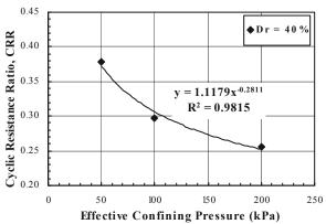
Figure 6. Variation of CRR with  $\sigma'_c$  for North Coast calcareous sand
