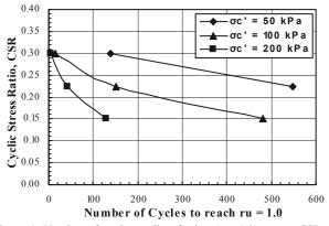
Figure 4. Number of cycles to liquefaction ( $r_u$ = 1.0) versus CSR at various  $\sigma'_c$  for North Coast calcareous sand ( $D_r$  = 40%)
