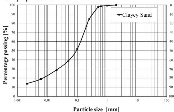
Figure 1. Grain size distribution of test material.
