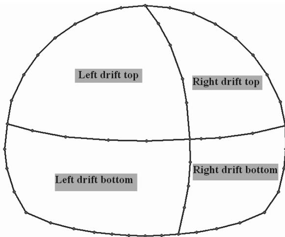
Figure 3. Stages of construction
