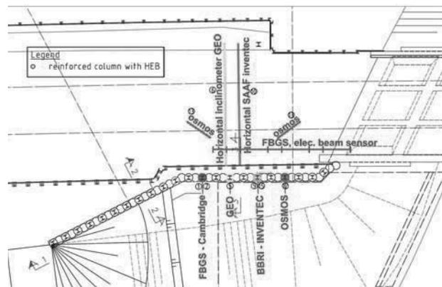
Figure 4. Top view of installed equipment.
