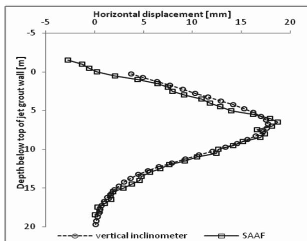
Figure 5. Horizontal deformation of the HEB profile on 07-03-2012.
