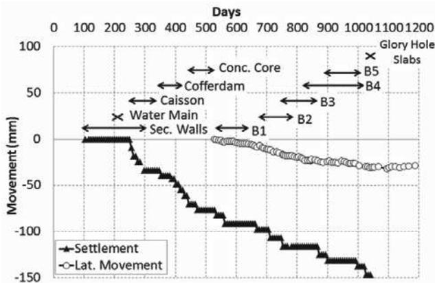
Figure 4. Settlements and lateral movements at OMPW
