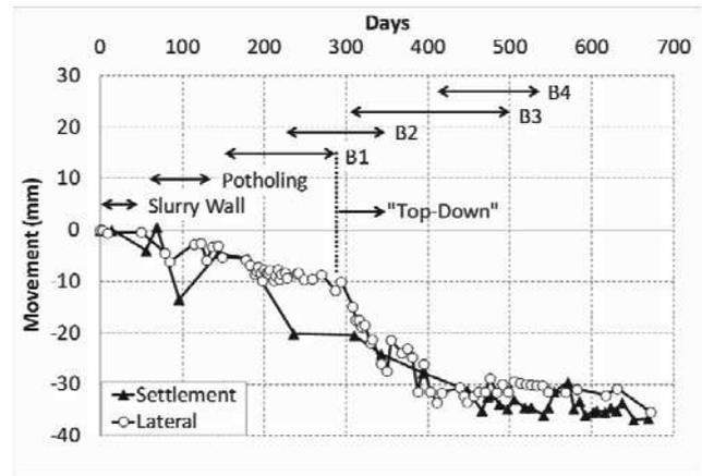
Figure 2. Settlements and lateral movements at Block 37
