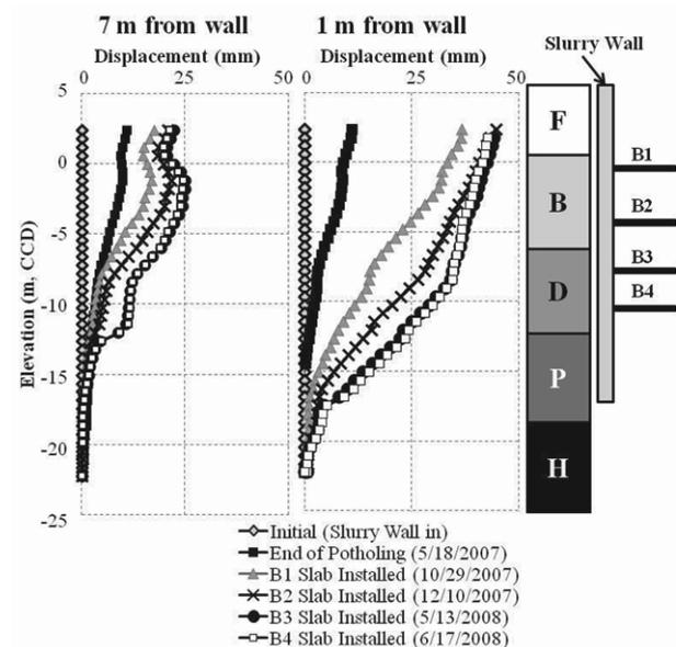
Figure 3. Lateral ground movements at Block 37
