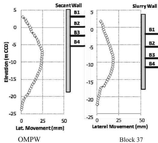
Figure 5. Lateral movements during top-down excavation only
