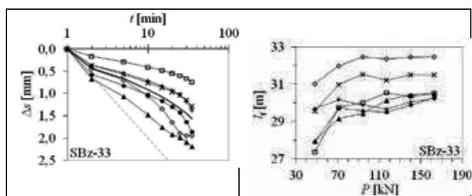
Figure 3. Measured increments of displacements of the anchor SBZ-33 (type RCP/D-I) at load level  $P_6$  of CST (left), apparent free lengths of individual strands  $l_f$  during CST (right).
