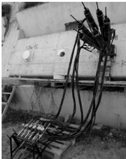
Figure 2. Test setup for simultaneous stressing of all strands of prestressed ground anchors using monostrand jacks.
