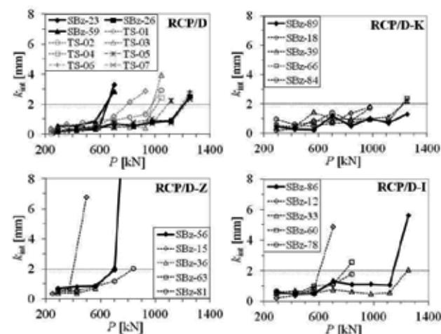
Figure 4. Interval creep displacement rates  $k_{int}$  for reference testing anchors as well as for all types of alternative anchors.
