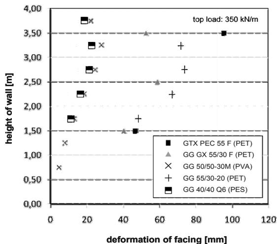
Figure 2. Deformation of full scale walls with semi-flexible facing, depending on the product (Pachomow & Herold, 2009).
