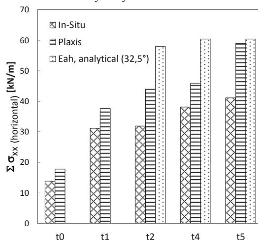
Figure 7. Comparison of measured lateral stress in situ, prediction by FE-analysis and prediction by classical earth pressure theory
