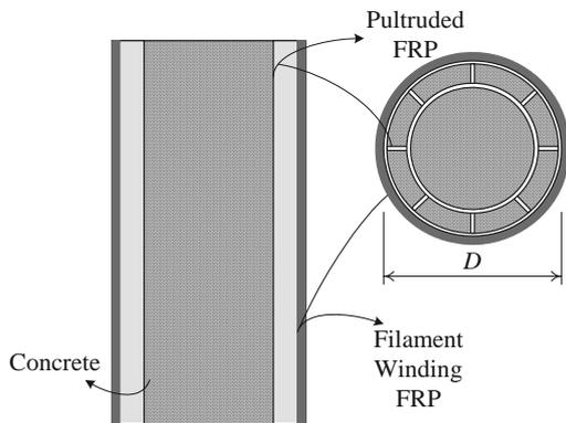
Figure 1 Hybrid FRP-concrete composite pile (HCFFP).
