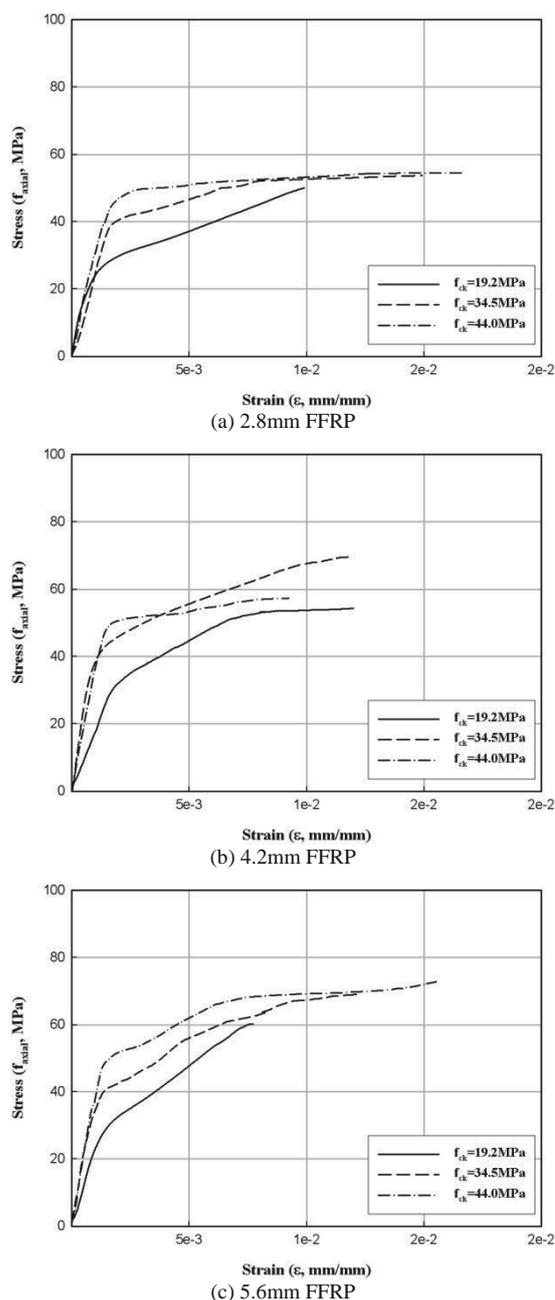
Figure 5 Axial stress-strain relationship of HCFFP specimen.
