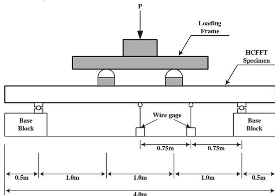
Figure 6 Loading and measurement location of HCFFP specimen.
