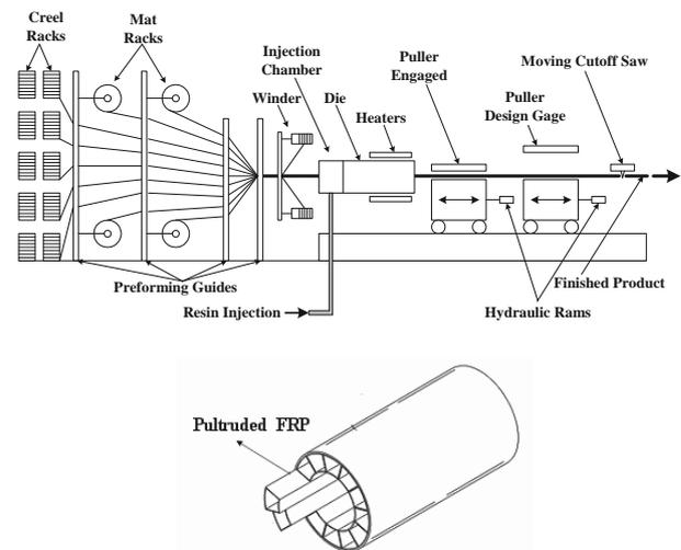
Figure 3 Manufacture of the pultruded FRP specimen.
