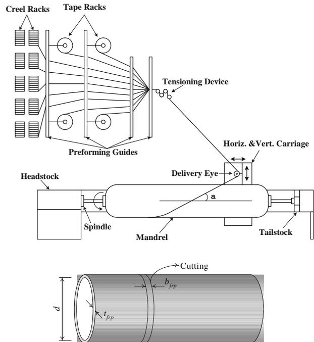
Figure 2 Manufacture of the filament winding FRP specimen.
