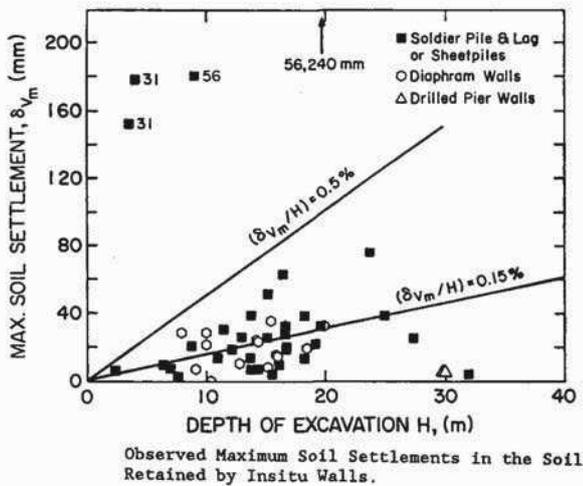
Figure 4 Observed maximum wall deflection and settlements for stiff clays, residual soils and sands (Clough and O'Rourke, 1990)
