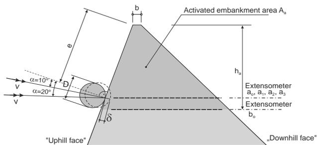
Figure 3. Model embankment system
