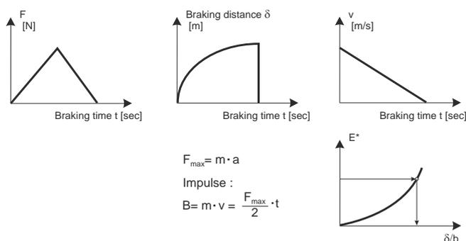
Figure 5. Assumptions for the evaluation (a = deceleration)
