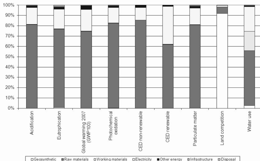
Figure 3. Environmental impacts of the life cycle of 1 kg geosynthetic layer. Geosynthetic includes direct burdens of the geosynthetic production. Raw materials include plastic, extrusion if necessary, and additives, working materials include water (tap and deionised) and lubricating oil, other energy includes thermal energy and fuels, infrastructure covers the construction of the production plant and disposal comprises wastewater treatment and disposal of different types of waste.
