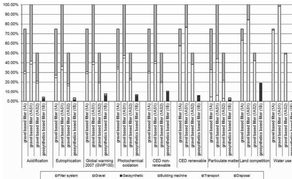
Figure 2. Sensitivity analysis: environmental impacts of the life cycle of 1 m<sup>2</sup> of filter layer. 1AS1 and 1AS2 refer to the sensitivity analysis with a different thickness of the gravel based filter layer. For each indicator, the case with highest environmental impacts is scaled to 100%.
