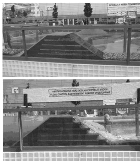
Figure 7. Model of reinforced dike before and after the test
