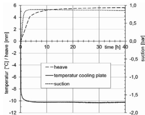
Figure 6. Development of suction and heave for kaolin due to drop of temperature of the cooling plate (surcharge 20 kN/m<sup>2</sup>, overconsolidated, closed system)
