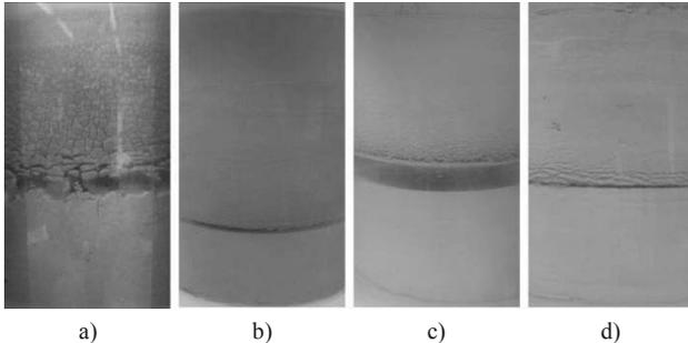
Figure 4. Specimens at the end of open system freezing tests: a) TS (100 kN/m<sup>2</sup>), b) S (20 kN/m<sup>2</sup>), c) K (20 kN/m<sup>2</sup>), d) K (100 kN/m<sup>2</sup>)
