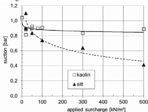
Figure 8. Dependency of the maximum suction on the applied surcharge
