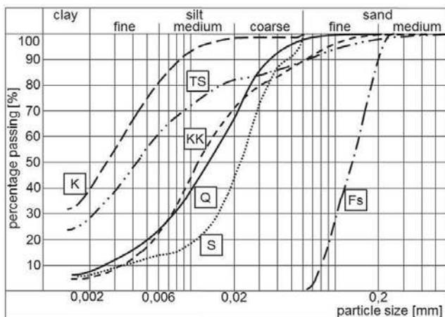
Figure 2. Grain-size distribution curve of the tested materials
