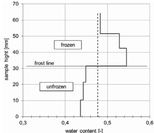
Figure 7. Water content distribution for a test with kaolin with an applied surcharge of 300 kN/m<sup>2</sup> (closed system)
