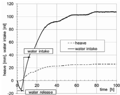
Figure 5. Changes in water content in the specimen and displacement with time for kaolin (20 kN/m<sup>2</sup>)
