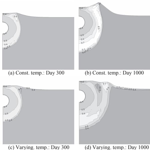
Figure 9. Computed geometry changes and porosity distributions.
