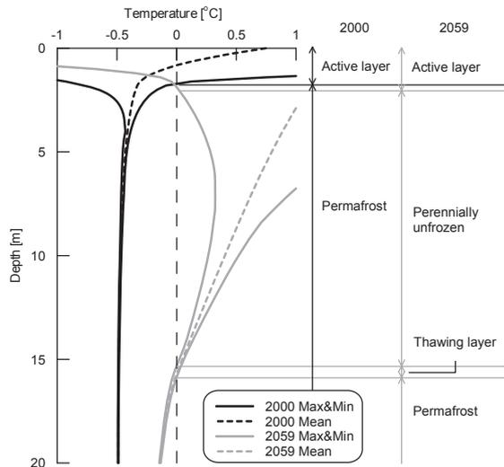
Figure 4. Computed annual temperature profiles for 2000 and 2059; Rolling Hills study area at 643mASL,  $n$ -factor = 0.6. Stratigraphy involves 1-m surface layer with porosity 0.4, decreasing to 0.04 at 15m depth.
