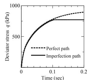
Fig. 10 Load control after displacement control ("creep")
