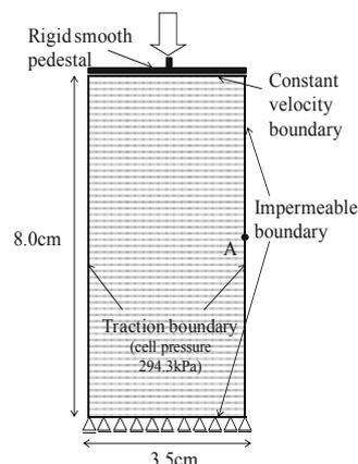
Fig. 1 Finite element mesh and boundary conditions
