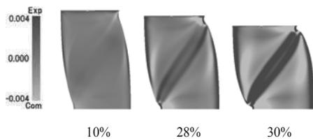
Fig. 14 Changes in specific volume (swelling shear bands)
