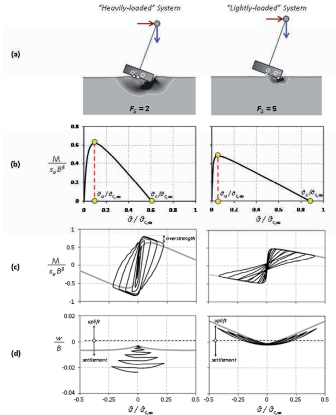
Figure 4. Comparison of two slender systems (differing only in  $F_S$ ) subjected to monotonic and cyclic loading: (a) deformed mesh with plastic strain contours at ultimate state; (b) dimensionless monotonic moment-rotation response; (c) cyclic moment-rotation response; and (d) cyclic settlement-rotation response (the grey line corresponds to the monotonic backbone curves).
