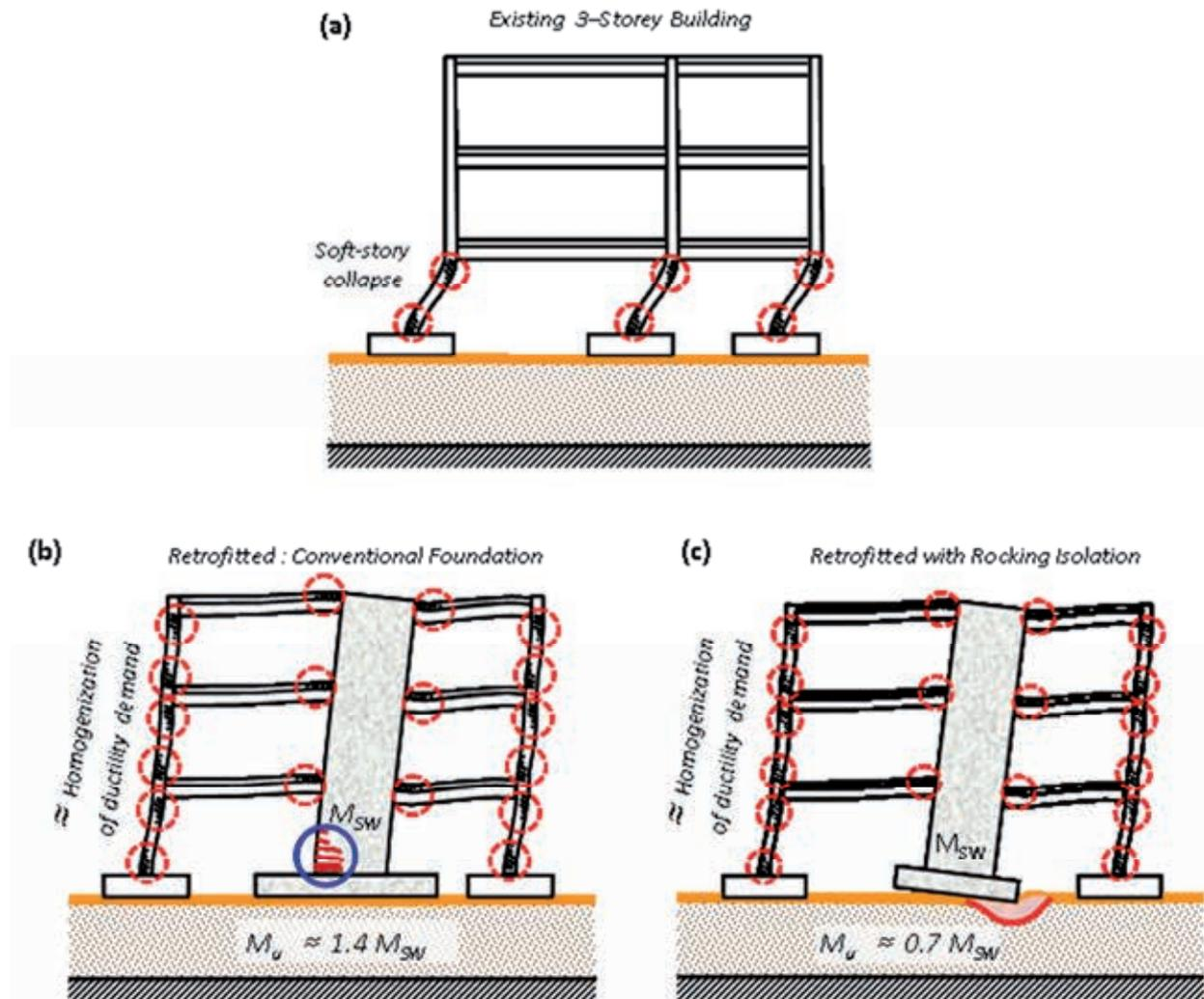
Figure 8. Sketches of damaged states of the three structures.
