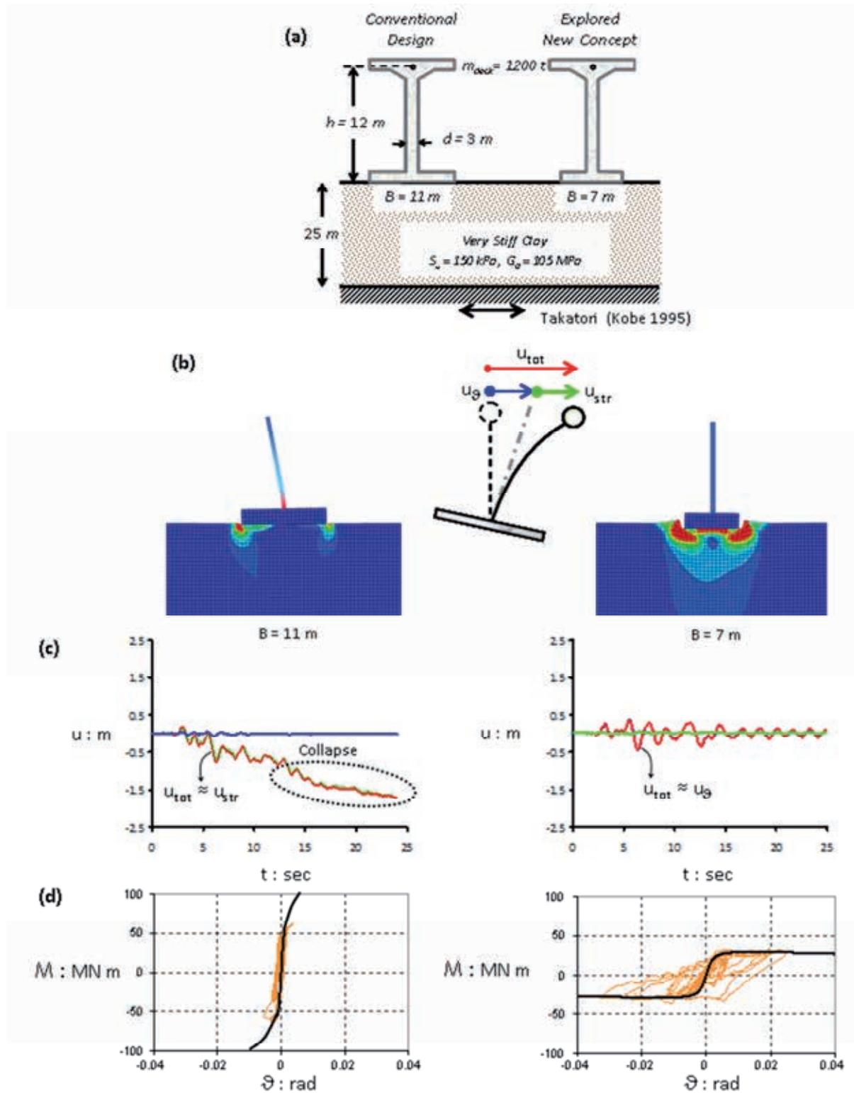
Figure 5. (a) Two bridge piers on two alternative foundations subjected to a large intensity shaking, exceeding the design limits; (b) deformed mesh with superimposed plastic strain, showing the location of “plastic hinging” at ultimate state; (c) time histories of deck drift; (d) overturning moment–rotation ( $M$ – $\theta$ ) response of the two foundations.
