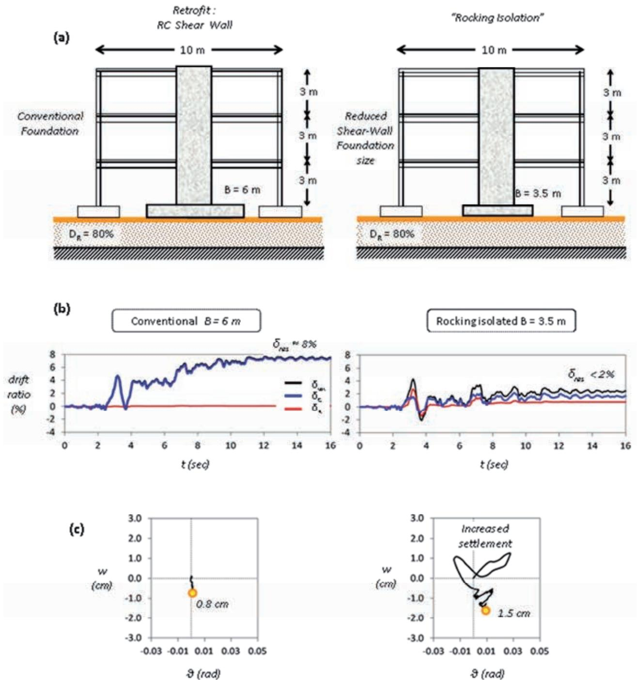
Figure 7. (a) Old frame retrofitted with stiff Shear Wall on two different foundations — conventional  $B = 6\text{ m}$  and unconventional  $B = 3.5\text{ m}$ ; (b) time histories on top floor drift ratio; (c) settlement-rotation curves of the Shear Wall footings.
