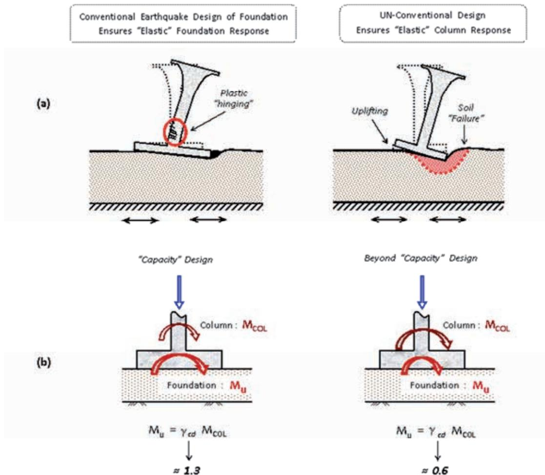
Figure 1. Conceptual illustration of (a) the response of a conventional and a "rocking-isolation" design of a bridge-pier foundation; and (b) the "capacity" design principle as conventionally applied to foundations, and its reversal in "rocking isolation".
