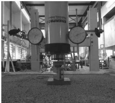
Figure 2. Experimental Setup with model footing, dial gauges and loading arrangement.
