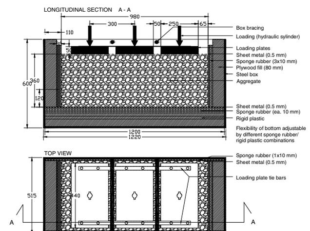
Figure 3. Test box prepared for cyclic loading tests.
