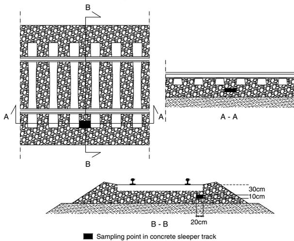
Figure 1. Sampling point of ballast bed samples.
