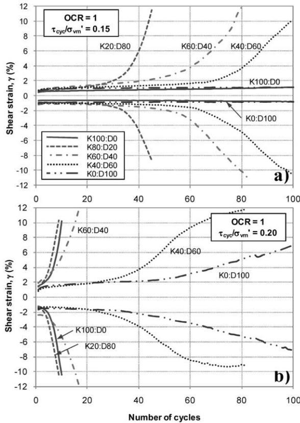
Fig. 3. Cyclic behavior of samples with OCR = 1 at different stress ratios a)  $\tau_{cyc}/\sigma_{vm}' = 0.15$  b)  $\tau_{cyc}/\sigma_{vm}' = 0.15$
