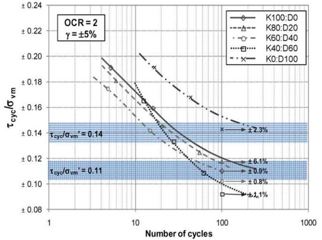
Fig. 6. Contour diagrams for samples with OCR = 2. Number of cycles to achieve  $\gamma = \pm 5\%$  for any cyclic shear stress.
