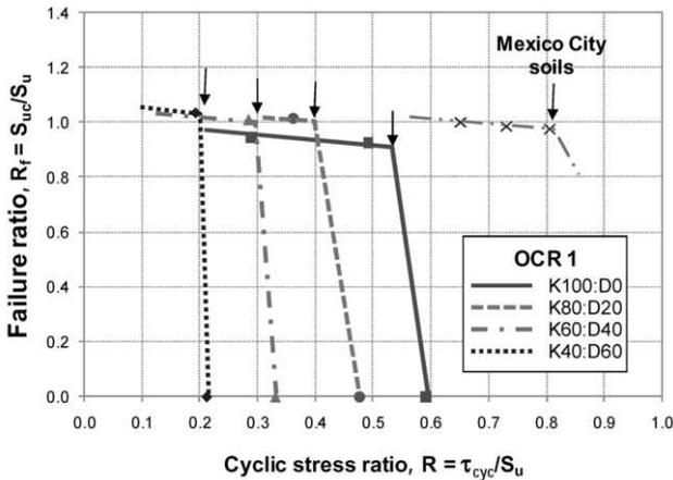
Fig. 7. Cyclic loading and residual undrained shear strength for samples with OCR = 1. Degradation threshold is indicated.
