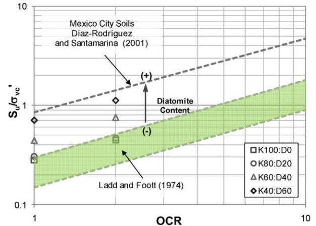
Fig. 2 Effect of OCR ( $\sigma_{vm}/\sigma_{vc}$ ) in undrained shear strength normalized with respect to effective confining stress
