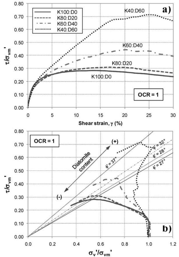
Fig. 1. Monotonic pre-cyclic behavior of samples with OCR = 1. a) Stress-strain curves b) Undrained stress paths.
