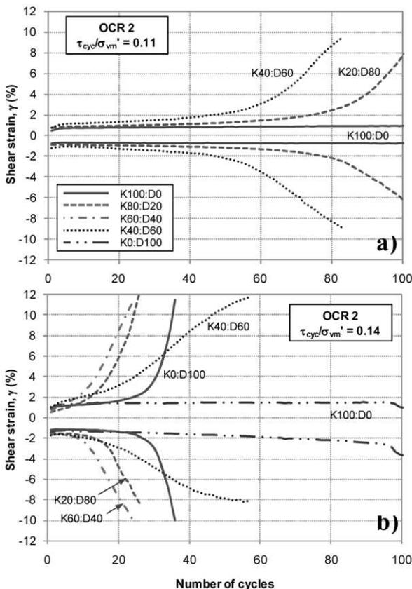
Fig. 4. Cyclic behavior of samples with OCR = 2 at different stress ratios a)  $\tau_{cyc}/\sigma_{vm}' = 0.11$  b)  $\tau_{cyc}/\sigma_{vm}' = 0.14$
