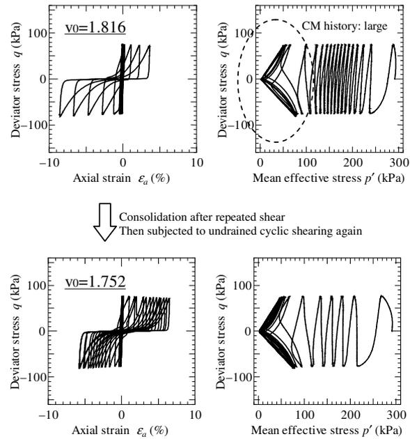
Figure 3. Reduction in liquefaction strength seen after reconsolidation
