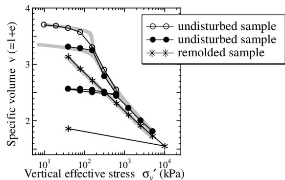
Figure 1. Standard consolidation test results
