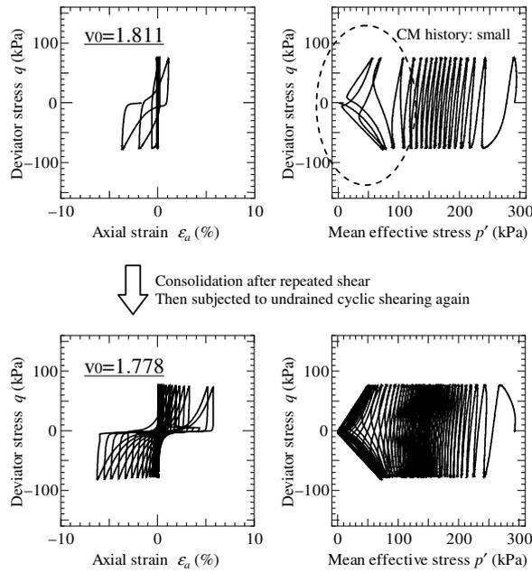
Figure 2. Increase in liquefaction strength seen after reconsolidation
