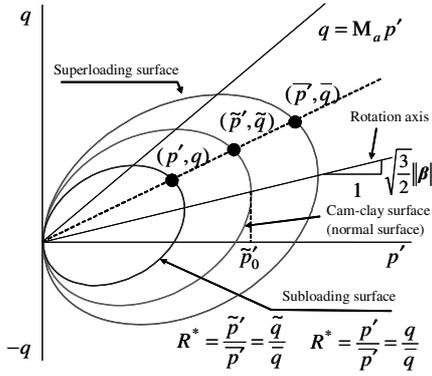
Figure 4. The three loading surfaces
