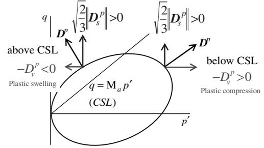
Figure 5. Sign of each component of plastic stretching
