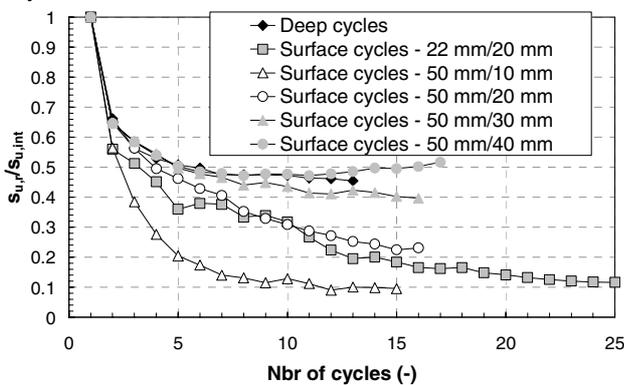
Figure 4. Strength loss at different depths in normally consolidated clay during deep and surface-breaking cyclic T-bar penetrometer tests.
