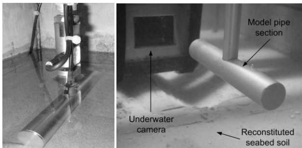
Figure 1. Arrangement of model pipe and loading arm
