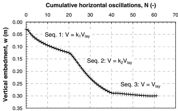
Figure 6. Dynamic lay simulation 1: Accumulation of pipe embedment
