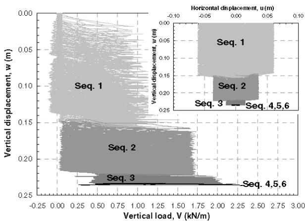
Figure 7. Dynamic lay simulation 2: Cyclic vertical loading and the associated pipe invert trajectory
