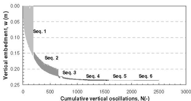
Figure 8. Dynamic lay simulation 2: Accumulation of pipe embedment
