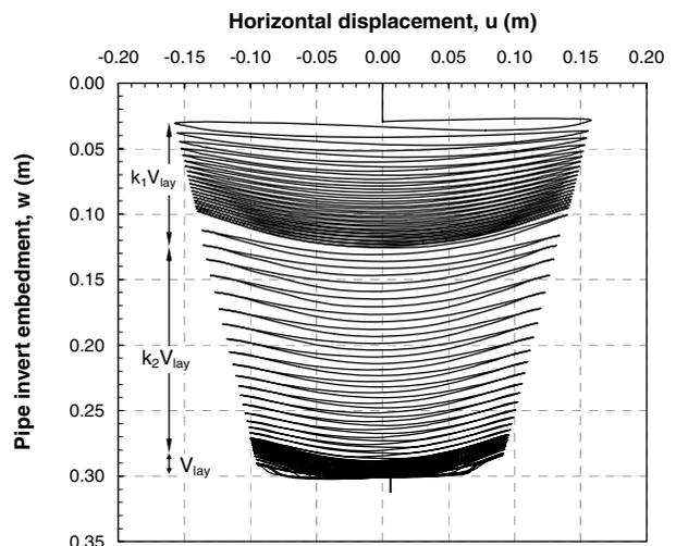
Figure 5. Dynamic lay simulation 1: pipe invert trajectory
