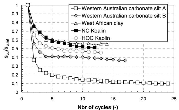
Figure 3. Degradation of strength during cyclic T-bar penetrometer tests.
