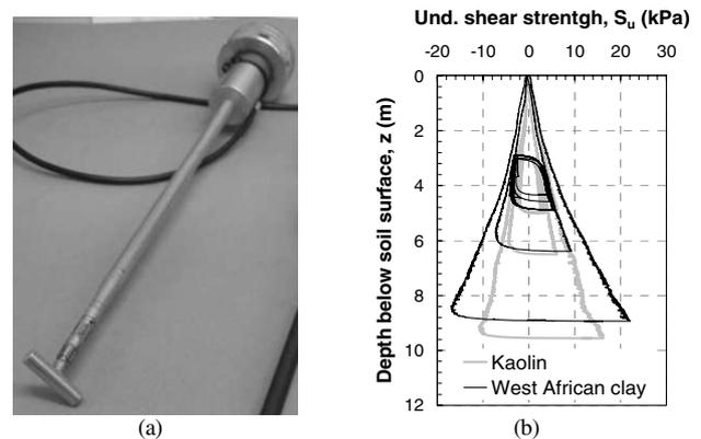
Figure 2. T-bar penetrometer used in the UWA beam centrifuge and typical undrained strength profiles from T-bar tests (depth in prototype scale units)
