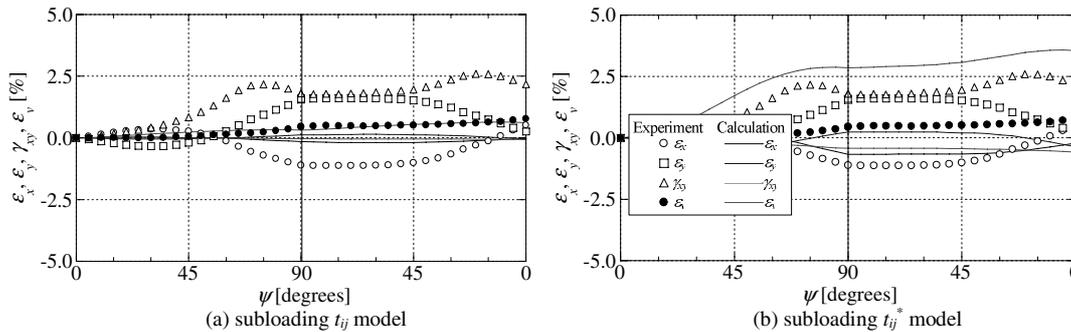
Figure 8. Directional shear cell test: Stress-strain relations of experiments and analysis (rotation of principal stress axes).
