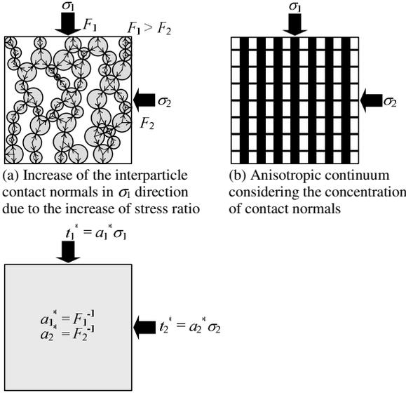
Figure 1. Modeling of induced anisotropy using modified stress.
