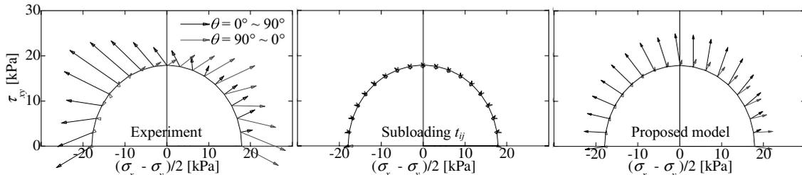
Figure 9. Directional shear cell test: Stress paths and strain increment vectors (rotation of principal stress axes).
