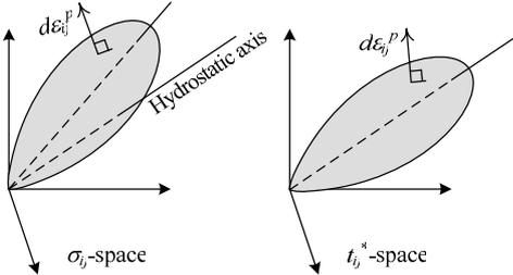
Figure 4. Comparison of the method for describing induced anisotropy.
