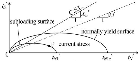
Figure 2. Yield surface on  $t_N^*$ - $t_S^*$  plane.
