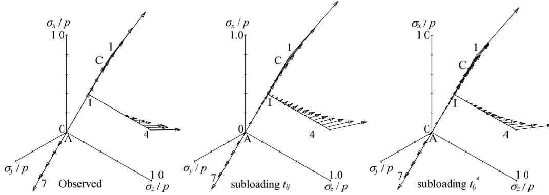
Figure 7. True triaxial tests: Stress paths and strain increment vectors (Stress paths ACI1, ACI4, ACI7)
