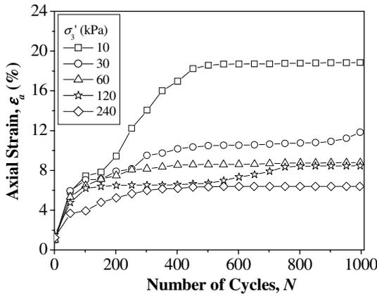
Figure 2. Variation of  $\varepsilon_a$  with  $N$  at different  $\sigma'_3$
