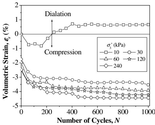
Figure 3. Variation of  $\varepsilon_v$  with  $N$  at different  $\sigma'_3$
