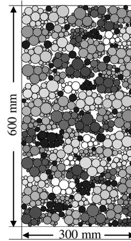
Figure 1. Initial assembly at  $\sigma'_3 = 10$  kPa
