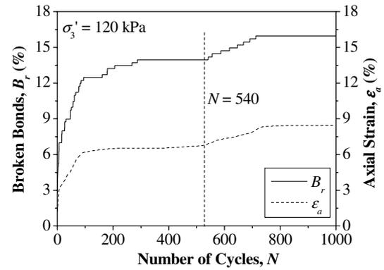
Figure 4. Effect of  $B_r$  on  $\varepsilon_a$  with  $N$
