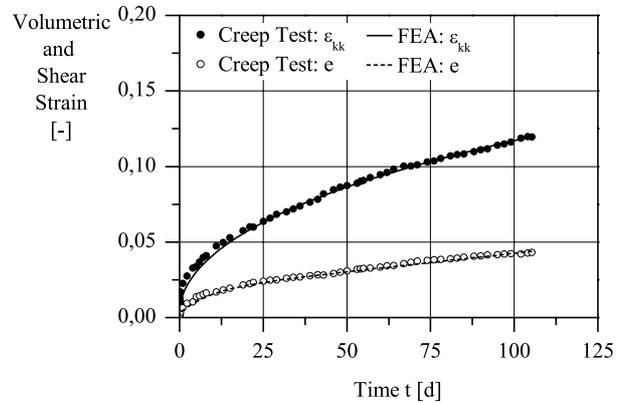
Figure 5. Simulation of a creep test.
