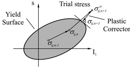
Figure 4. Pattern of the return-mapping-algorithm.
