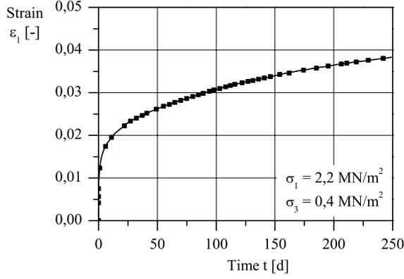
Figure 2. Triaxial creep test.
