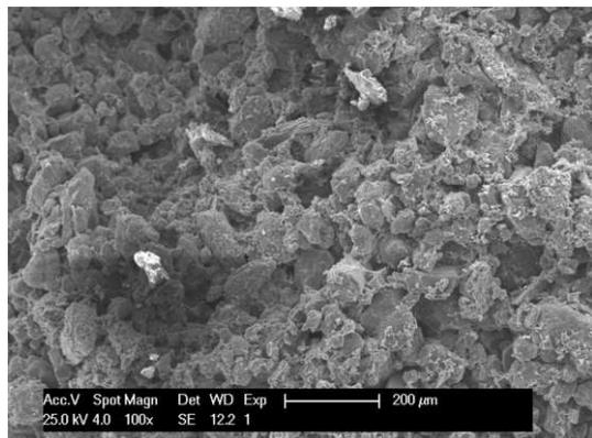
Figure 2. Loess sample before collapse; 100x magnification
