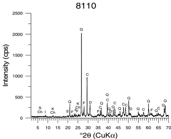
Figure 5. X-ray diffractometrical analysis of loess (sample: 08-110)
