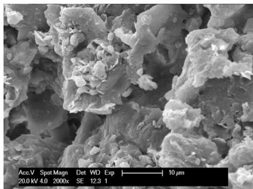
Figure 4. Loess with high salt and lime contents, 2000x magnification
