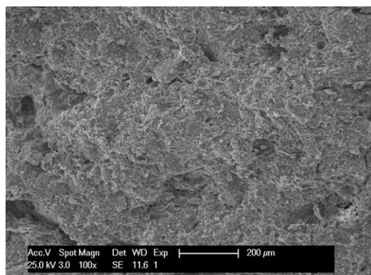
Figure 3. Same loess sample after collapse; 100x magnification
