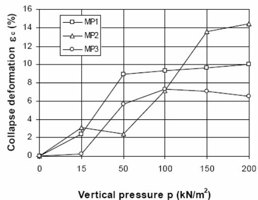
Figure 1. Collapse deformation of loess samples
