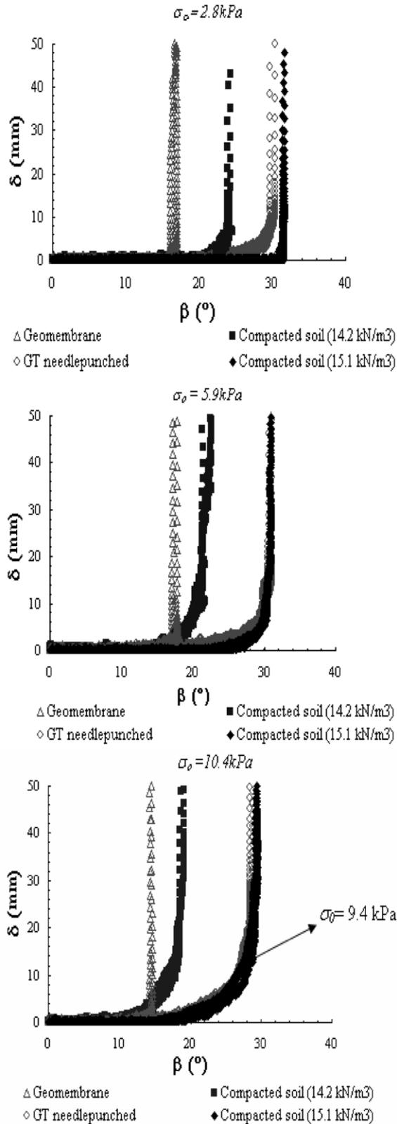
Figure 3. Displacement  $\delta$  versus inclination  $\beta$  relationships.
