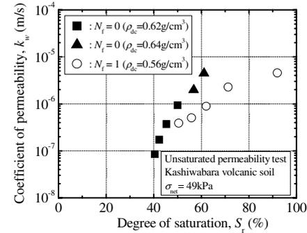
Figure 8. Comparison of coefficient of permeability.
