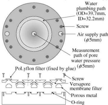
Figure 3. Structural design of cap and pedestal.
