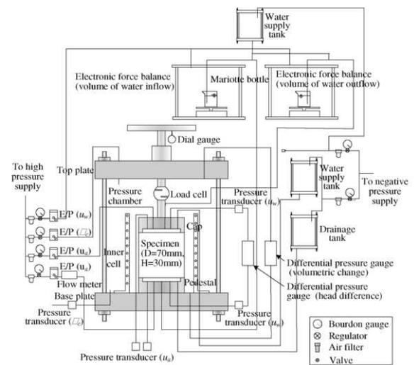
Figure 2. Freeze-thawing permeability test apparatus.
