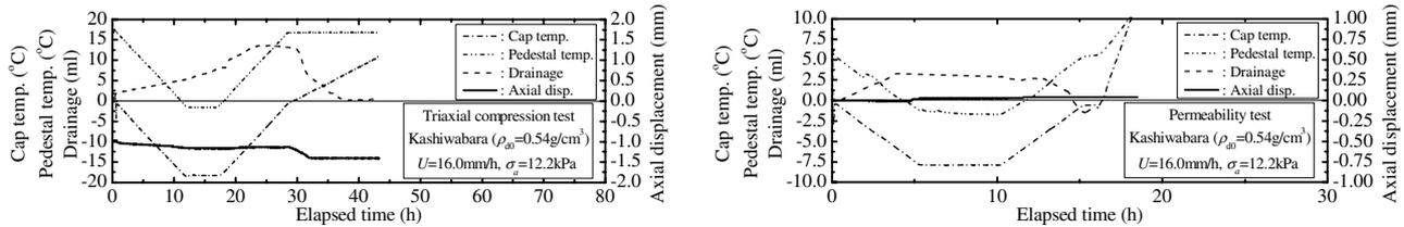
Figure 5. Comparison of frost heave behaviors between samples.
