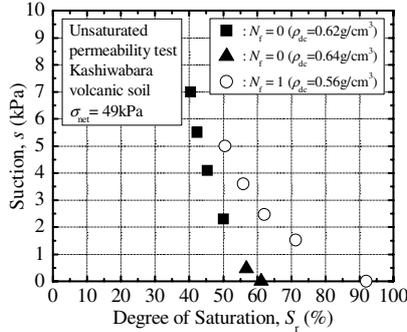
Figure 7. Comparison of water retention curves.
