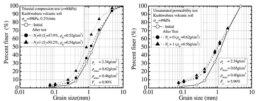
Figure 4. Grain size distribution of samples.
