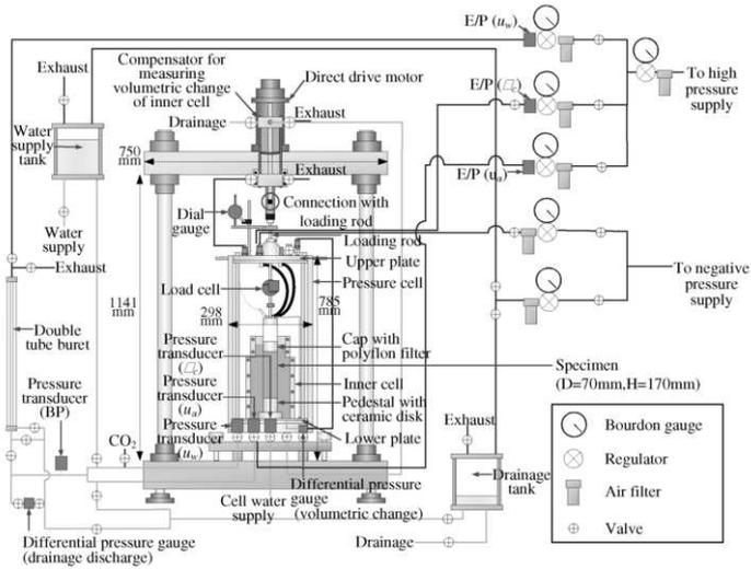
Figure 1. Freeze-thawing triaxial test apparatus.
