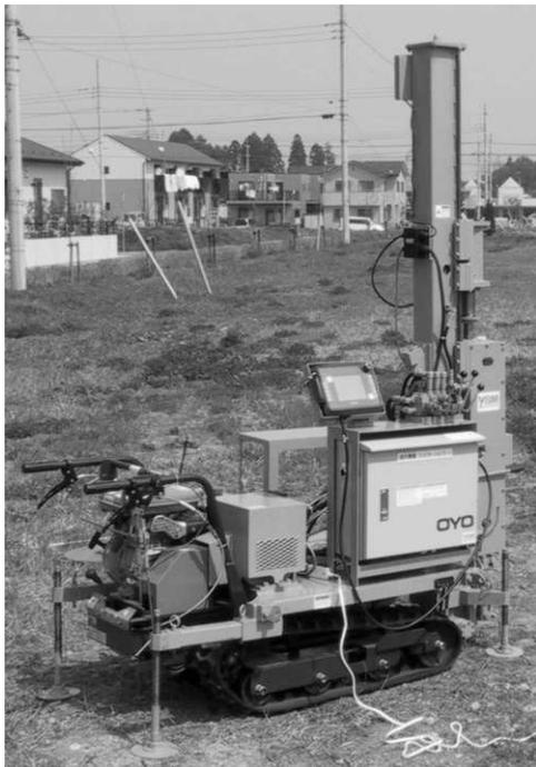
Figure 1. New combination cone penetration equipment.
