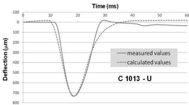
Figure 8. Comparison between calculated and measured values of deflection curve (5<sup>th</sup> drop at C 1013 location, U station).
