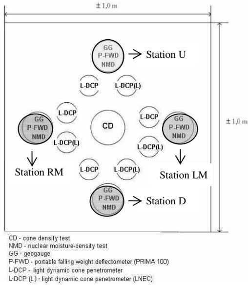
Figure 1. Field tests performed at each location.
