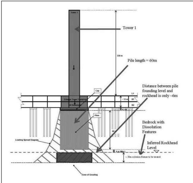
Figure 6. Simplified Load Spread Diagram of Tower 1
