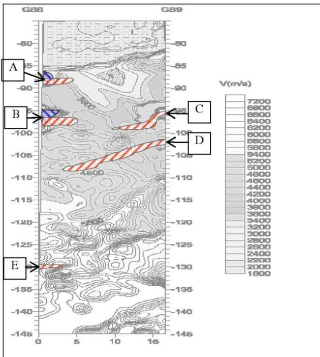
Figure 5. Comparison of Results of EM-Wave and Seismic-Wave CT Methods
