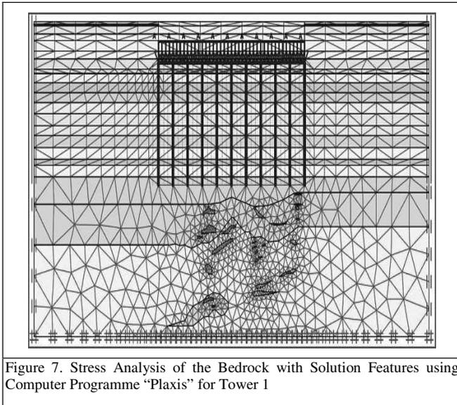
Figure 7. Stress Analysis of the Bedrock with Solution Features using Computer Programme "Plaxis" for Tower 1
