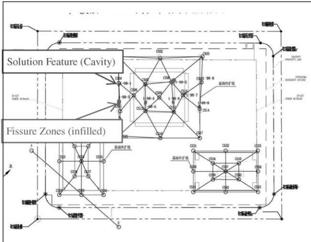
Figure 3. Plan Imaging of Seismic Wave CT Method of Tower 1 at Level -98mPD
