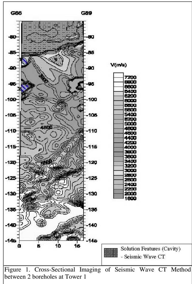
Figure 1. Cross-Sectional Imaging of Seismic Wave CT Method between 2 boreholes at Tower 1
