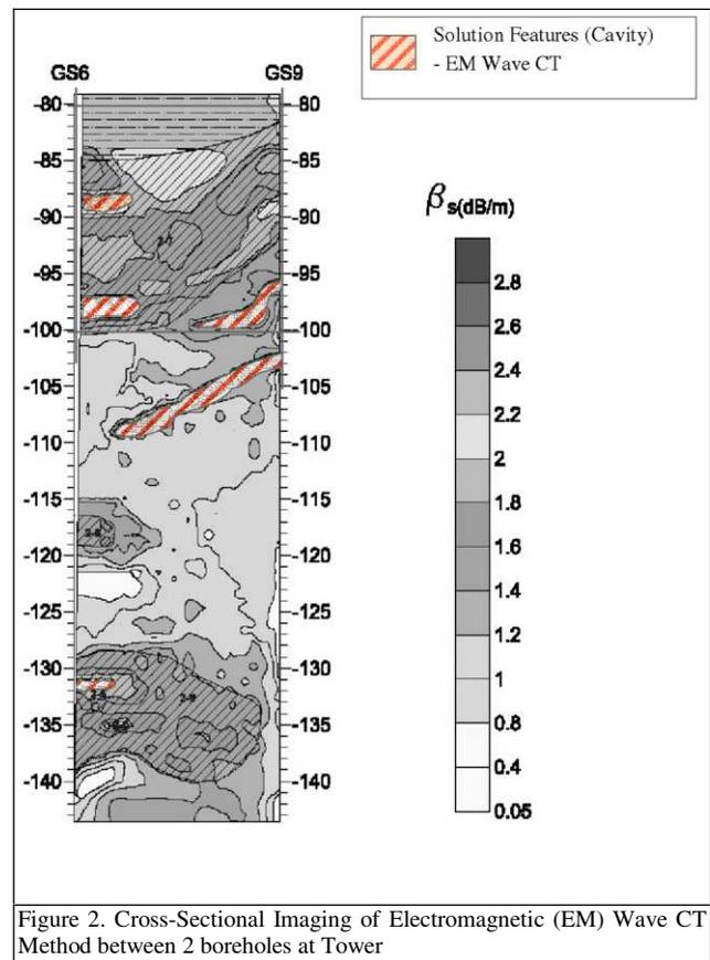
Figure 2. Cross-Sectional Imaging of Electromagnetic (EM) Wave CT Method between 2 boreholes at Tower 1
