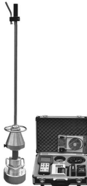
Figure 1. The B&C small-plate device
