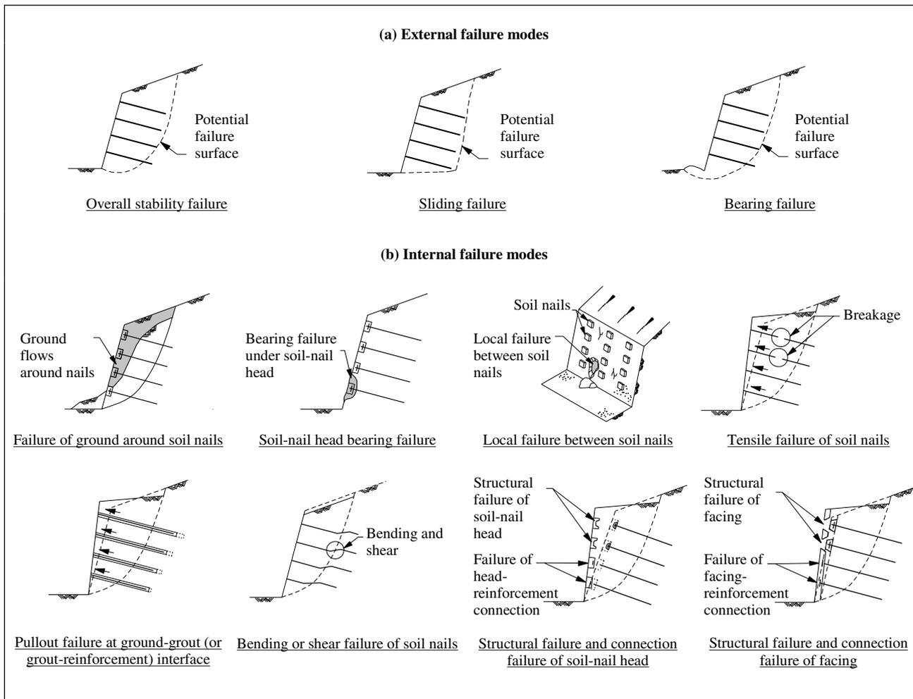
Figure 1. Potential failure modes of a soil-nailed system
