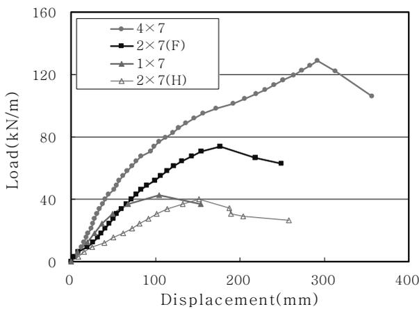
Figure 6. Pull-out behavior of Tirecell for different length
