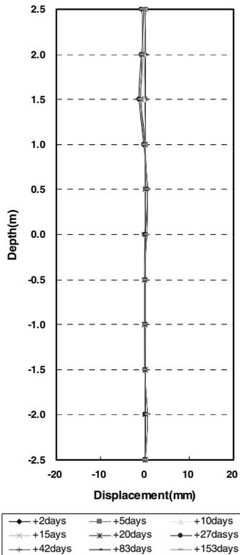
Figure 9. Lateral displacement of the retaining wall
