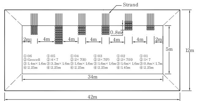
Figure 4. Field pull-out testing program for various conditions
