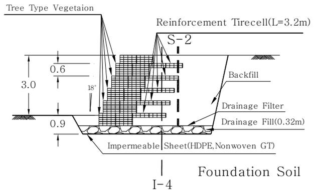
Figure 8. Schematic diagram of Tirecell reinforced retaining wall
