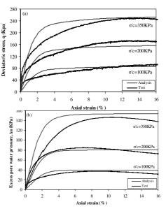
Figure 1. Tests and analyses results of T100 specimen: (a) deviatoric stress, and (b) excess pore water pressure.
