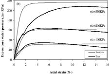
Figure 2. Tests and analyses results of ST40 specimen: (a) deviatoric stress, and (b) excess pore water pressure.
