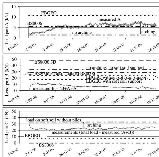
Figure 3. Comparison of measurements in the Kyoto Road and predictions with EBGEO and BS8006
