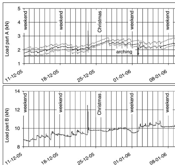
Figure 4, detail of Kyoto Road measurements. The arching is reduced due to the truck passages, but during rest periods (weekends, Christmas), the arching restores and develops further.
