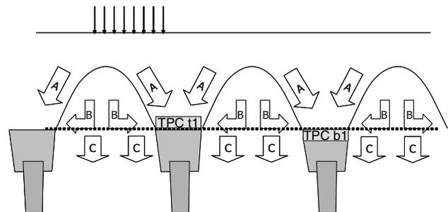
Figure 1. Load distribution into load parts A, B and C. Locations of Total Load Pressure Cells (TPC's) in the Kyoto Road field test
