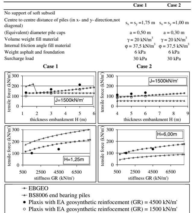
Figure 2. Tensile forces in the geosynthetic reinforcement (GR), for the case study for case 1 and case 2.
