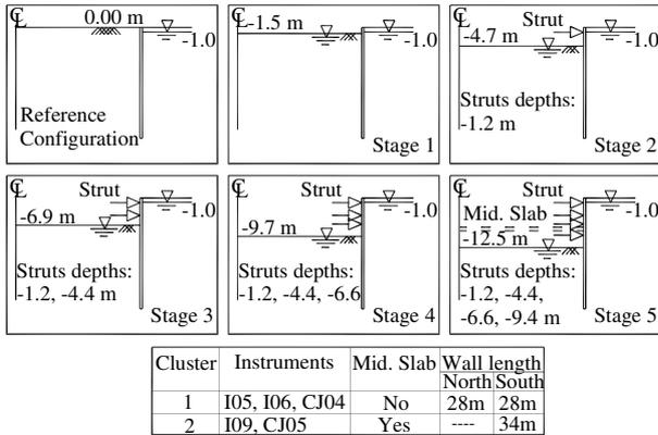
Fig. 4. Construction sequence for different clusters
