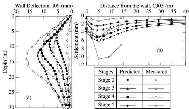
Fig. 7. Predicted deformations in cluster 2 after six passes of SelfSim learning with Cluster 1 deformations; a) wall deformations (109) and b) surface settlement CJ05, (middle slab was used)
