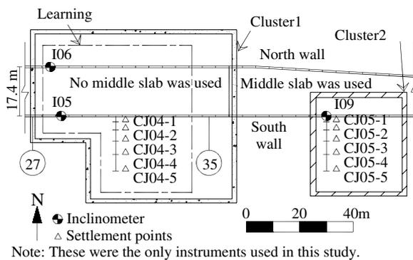
Fig. 2. Plan view of Yishan road metro station and instrument locations, Shanghai excavation, modified after Liu et al. (2005)
