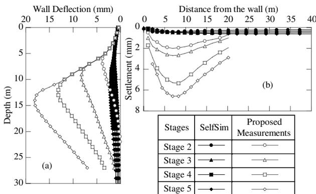
Fig. 5. Computed deformations in Cluster 1 prior to SelfSim learning; a) wall deformations, and b) surface settlements
