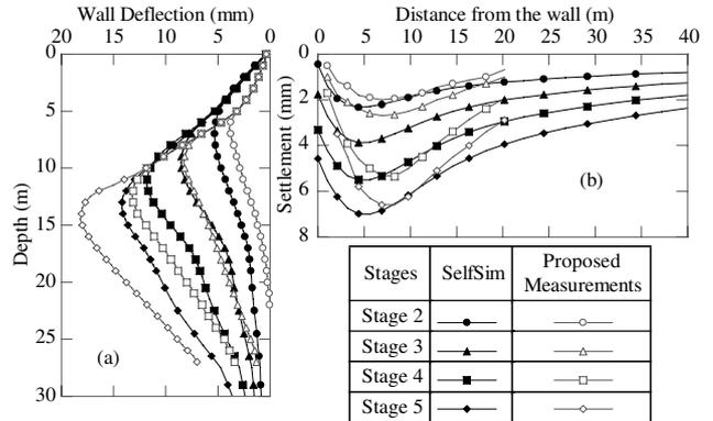
Fig. 6. Computed deformations in Cluster 1 after six passes of SelfSim learning with Cluster 1 measured deformations; a) wall deformations, and b) surface settlements
