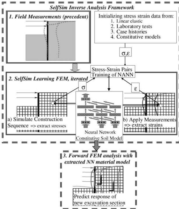
Fig. 1. Application of SelfSim inverse analysis framework to predict ground response at a new excavation section or site
