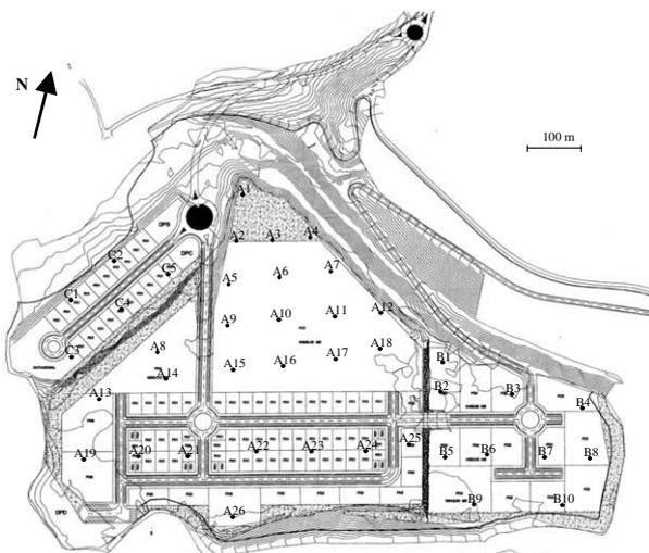
Figure 3. Reference points for control of settlements
