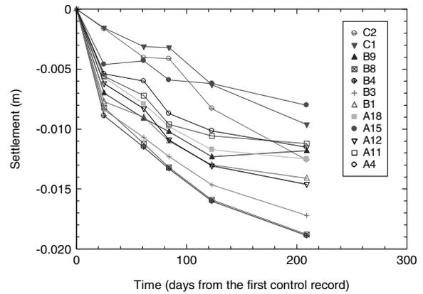
Figure 5. Settlement records in the upper platform (zones A, B and C)
