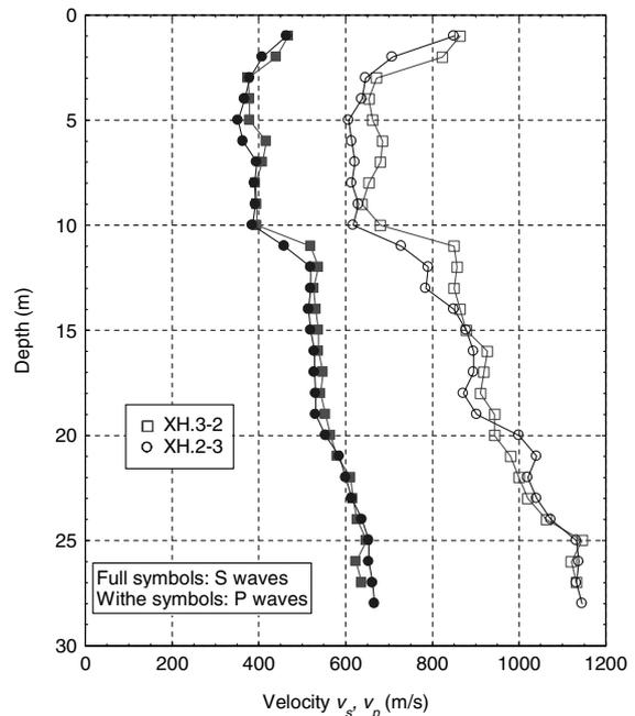
Figure 4. Cross-hole tests results between S2 and S3
