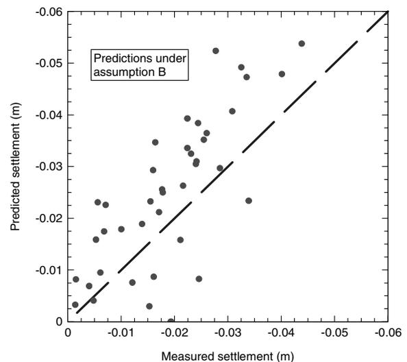
Figure 7. Measured and predicted (assumption B) settlements at 902 days
