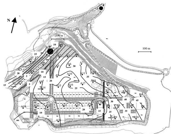
Figure 6. Predicted settlement (cm) for t=25 years (assumption A)
