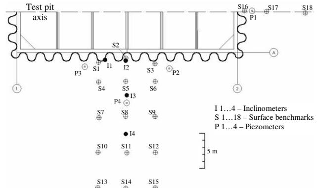
Figure 5. Position of monitoring equipment near the test pit.
