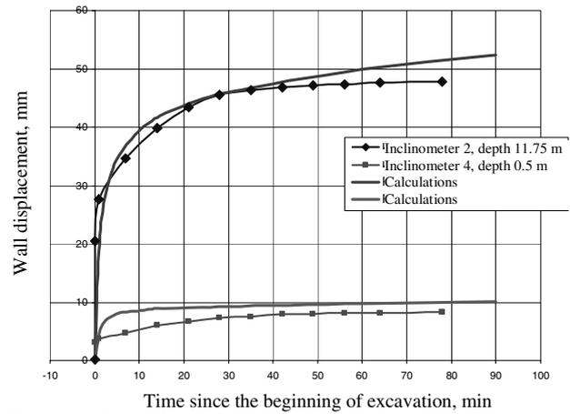
Figure 8. Comparison of the deformations development in various locations of the soil with the calculations made with the Visco-elasto-plastic model.
