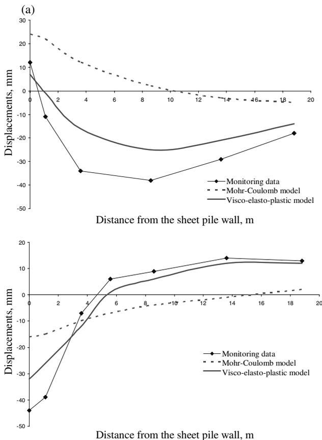
Figure 7. Comparison of vertical (a) and horizontal (b) displacement of the benchmarks as obtained during monitoring and as was predicted by calculations using different models.
