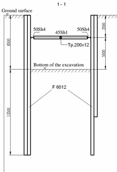
Figure 3. Cross-section of the excavation at the test pit.
