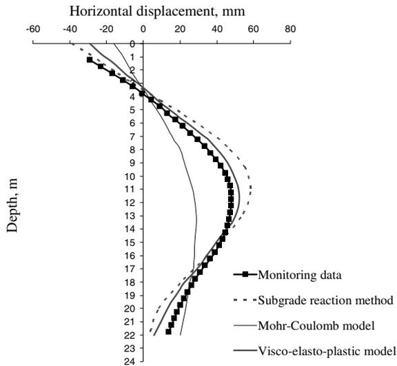
Figure 6. Comparison of the monitoring data of the cofferdam movements with the calculations based on various models.
