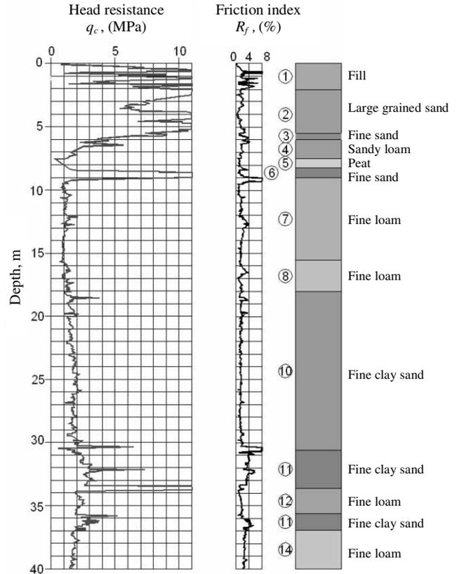
Figure 4. Geotechnical profile and results of SPT test carried out at the test pit.
