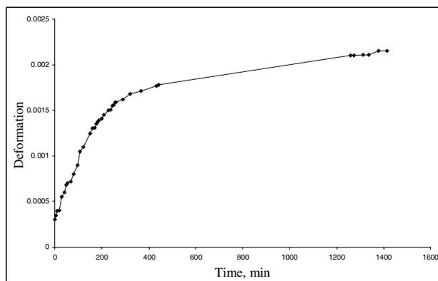
Figure 1. Unconfined creep test of the undisturbed sample of liquid loam at constant vertical normal stress of 5.4 kPa.
