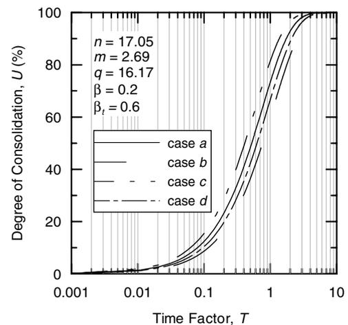
Figure 3. Plots of degree of consolidation versus time factor for different hydraulic conductivity profiles.
