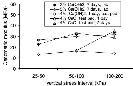
Figure 7. Oedometer modulus measured on samples compacted in the laboratory and taken from the test pad (curing times in the legend).
