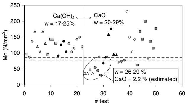
Figure 10. Soil-lime mixture modulus,  $M_d$ , measured by PLT on the embankments during construction (curing times: 1-3 weeks; pressure: 150-250 kN/m<sup>2</sup>). The sequence of tests follows the construction sequence (symbols mark different embankments portions).
