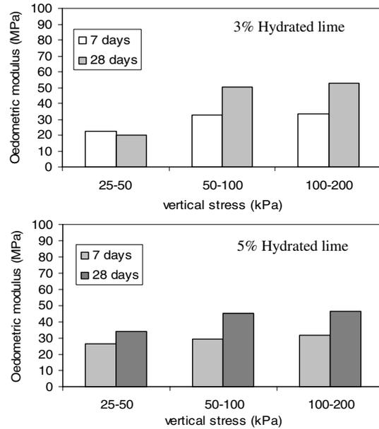
Figure 3. Results of oedometer tests on the soil-hydrated lime mixtures at different curing times (in the legend), all compacted at  $w_{opt} \pm 2\%$ .
