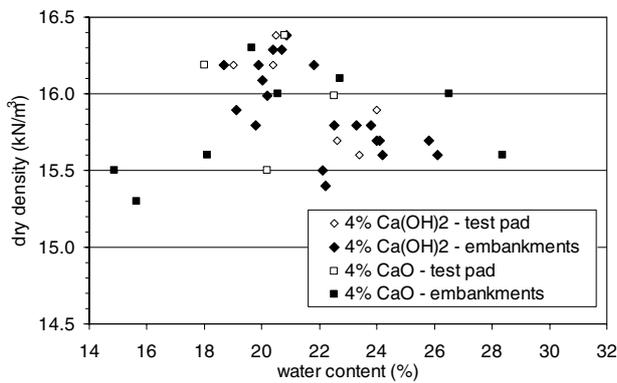
Figure 8. Dry density of the soil-lime mixtures during construction compared with the dry density of the samples from the test pad.
