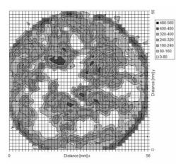
Figure 9. Stress distribution at displacement of 18 mm in the test 3.2\_dtv model A
