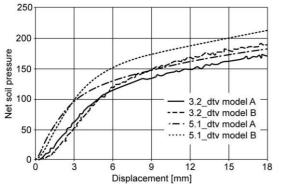
Figure 8. Net soil pressure-displacement curves for foundations tested after dynamic compaction
