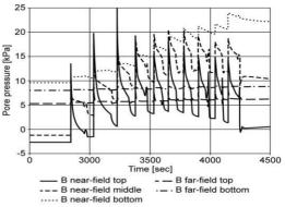
Figure 7. Pore pressure variations during 10 impact events for 3.2\_dtv model B, with nominal 2.7 kJ impact energy
