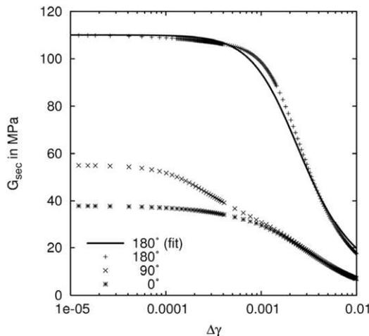
Figure 1. Calculated secant stiffness for a biaxial compression with constant volume after a change of strain path direction.
