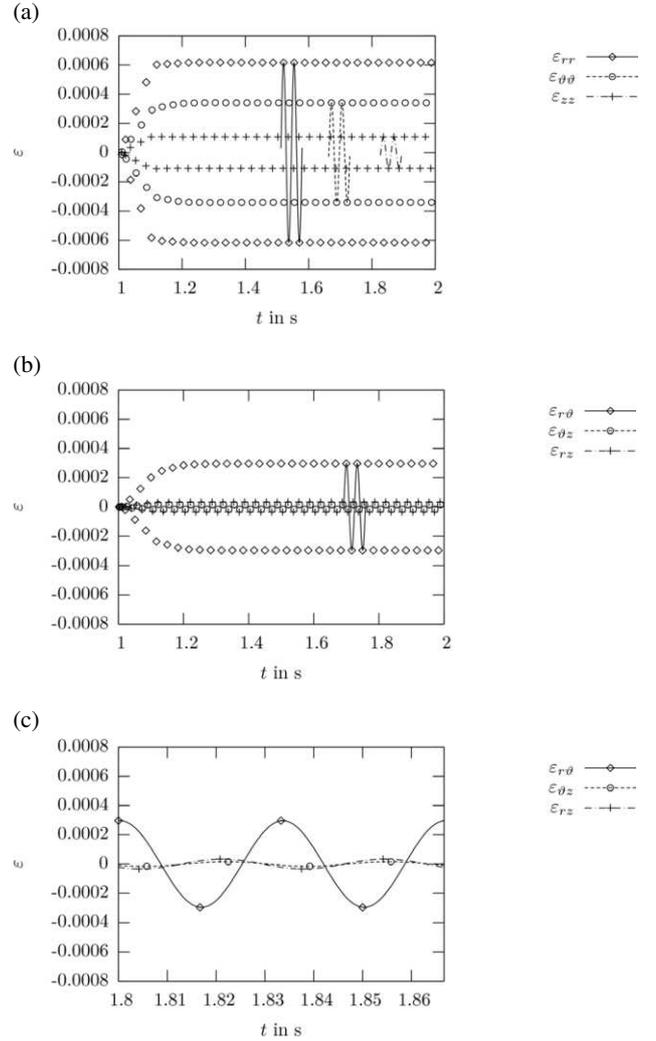
Figure 4 (a) Envelope of maximum normal strains, (b) envelope of maximum shear strains and (c) shear strains of two selected cycles at a distance 2.8 m from the symmetry line in the deep vibrator problem.
