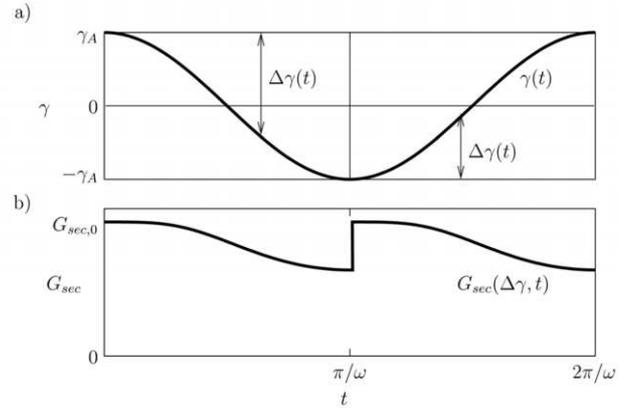
Figure 2. a) Shear strain vs. time, b) secant shear modulus vs. time during one strain cycle.
