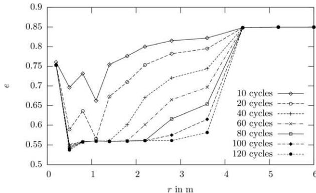
Figure 6. Evolution of void ratio along radial distance from the vibrator.
