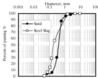
Figure 1. Particle size distribution curve for tested sand and steel slag.
