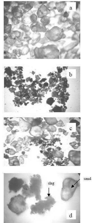
Figure 2: Microstructures of tested samples with magnification X100. a- Sand samples. b- Steel slag sample. c- Sand mixed with slag. d- Slag and sand with magnification X200.
