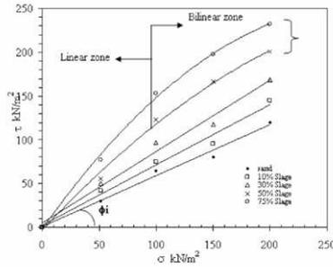
Figure 9: Strength envelopes for sand reinforced with varying slag content.
