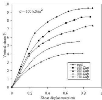
Figure 4. Relationship between vertical strain and shear displacement for different slag percentages
