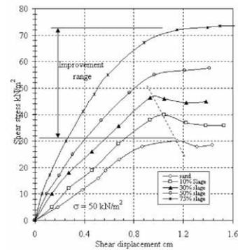
Figure 7. Shear stress versus shear displacement for different slag percentages.
