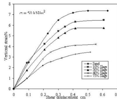
Figure 3. Relationship between vertical strain and shear displacement for different slag percentages.
