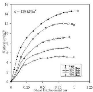
Figure 5: Relationship between vertical strain and shear displacement for different slag percentages.
