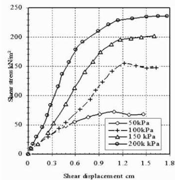
Figure 8: Shear stress versus shear displacement at different vertical confining pressure (Slag content 75%).
