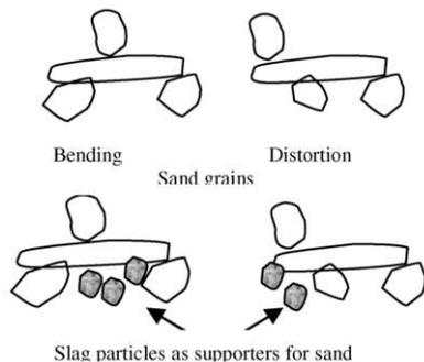
Figure 11: Interconnecting supports and failure mode.
