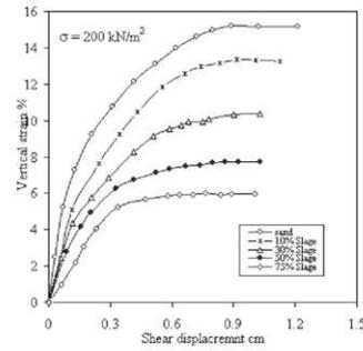
Figure 6. Relationship between vertical strain and shear displacement for different slag percentages.
