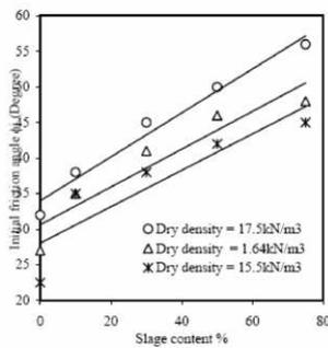
Figure 10. Initial friction angle versus slag content ( $\gamma_{Dry} = 17.5 \text{ kN/m}^3$ ).
