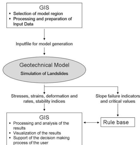
Figure 1. System architecture of the coupled system
