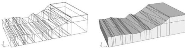
Figure 2. Wire-frame model for a section of a slope as basis for the set-up of a geotechnical model (transparent and shaded)
