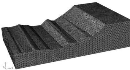
Figure 3. FE-mesh on the wire-frame model from Figure 2
