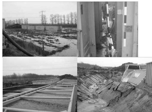
Figure 13. a) Overview preliminary test b) Measurement row at the centre of the container row c) Filling of the containers d) Failure
