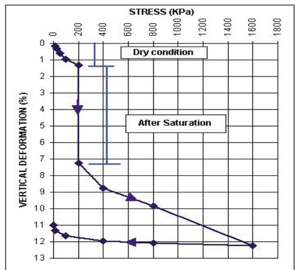
Fig. 5 Oedometer test on saline sample before and after saturation
