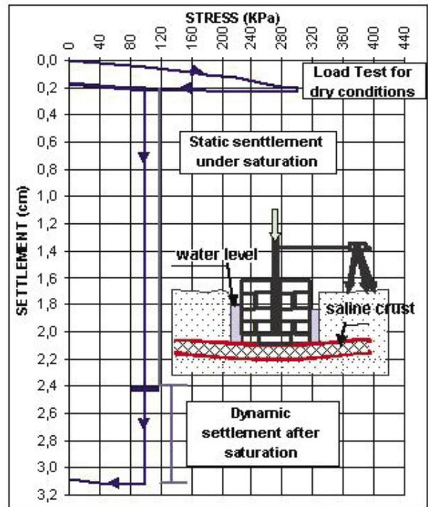
Fig.4 Settlement in load test before and after saturation.
