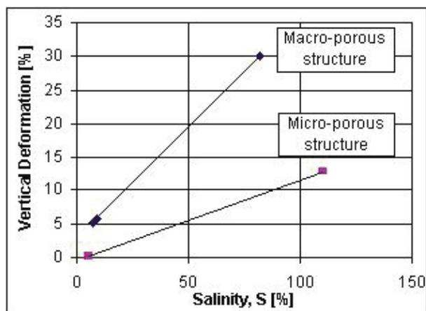
Fig. 6 Influence of structure on deformation after saturation in oedometer tests.
