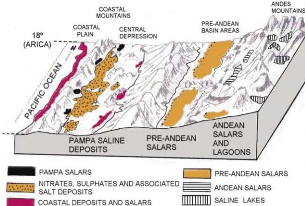
b. Schematic profile of distribution of saline soils in longitudinal bands.
