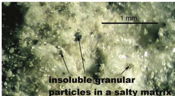
Fig. 3 Micro-porous structure
