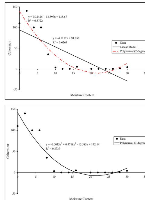
Figure 1: Cohesion - Moisture Models (Raw Data) For Sample 1
