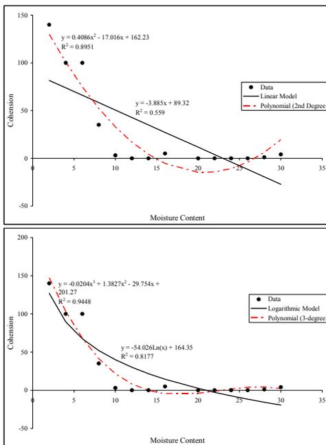
Figure 2: Cohesion - Moisture Content Models (Modified data) for Sample 1
