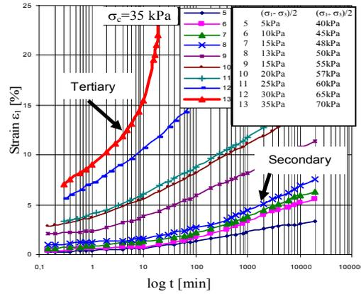
Figure 7. Strain versus log time for consolidated peat.
