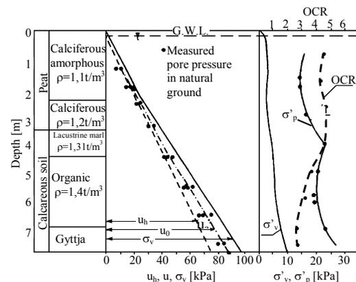
Figure 1. Geotechnical conditions in organic subsoil.
