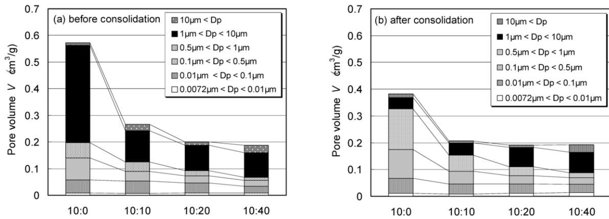
Figure 9. Pore entrance size frequency (a) before consolidation test and (b) after consolidation test
