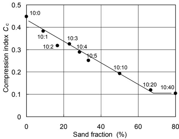
Figure 5. Relationships between compression index and sand fraction
